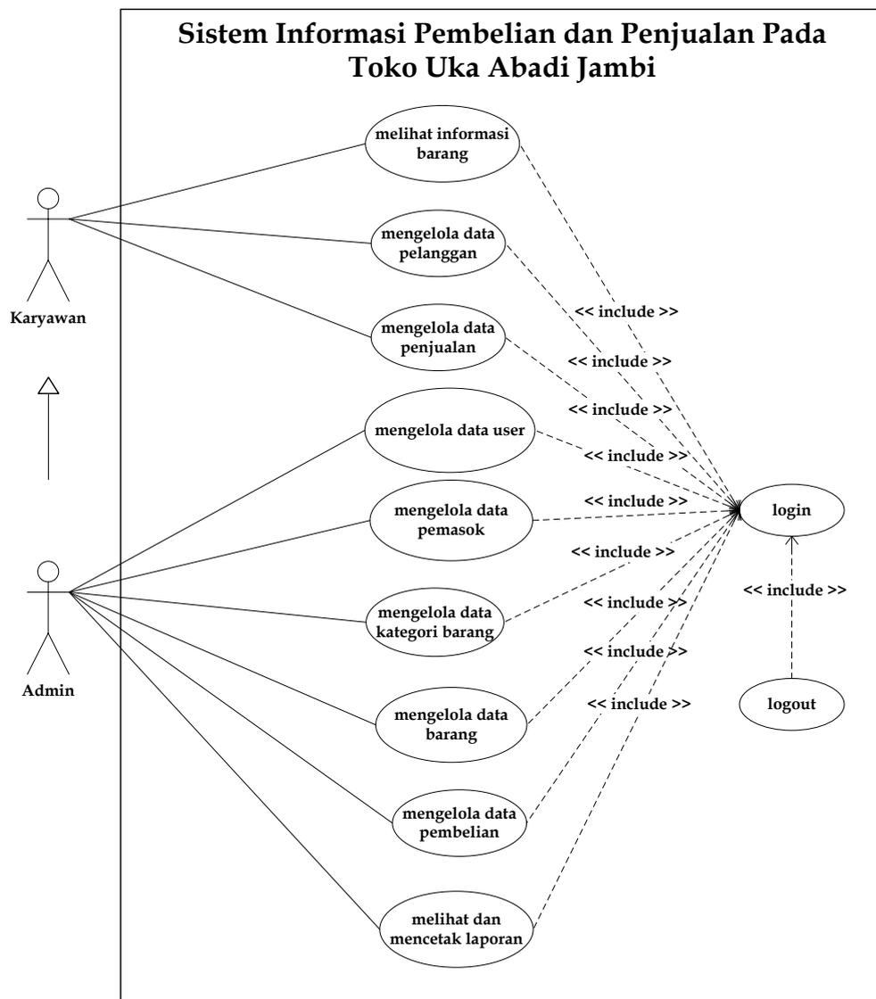
**Gambar 4.3 Use Case Diagram**
